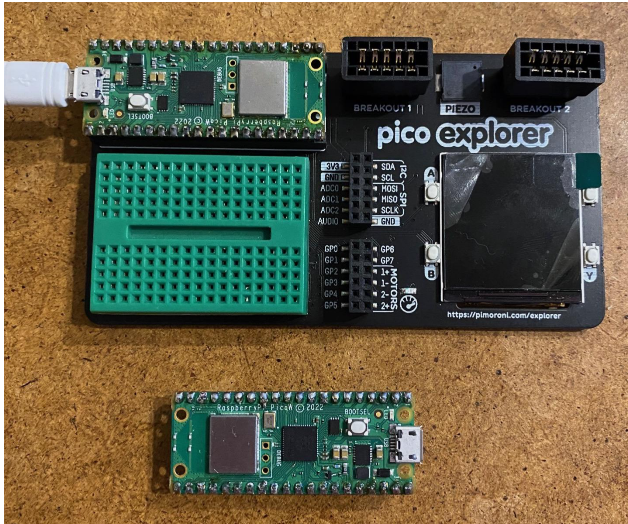
Figure 1 - A Raspberry Pi Pico W by Itself and Mounted in an Explorer Board
