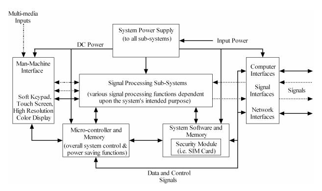
Figure 1 – Block Diagram of a typical modern electronic system (showing typical system sub-systems and the interconnections between them)
