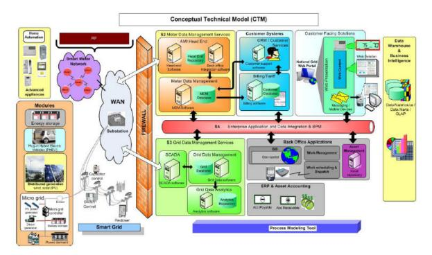
Figure 3 – Conceptual technical model of the Smart Grid (Source National Grid - Proposal submitted to Rhode Island Public Utilities Commission – Smart Grid Pilot Program<sup>9</sup>)
