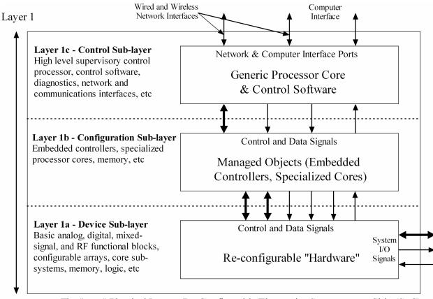
The "new" Physical Layer - Re-Configurable Electronics Systems on a Chip (SoC)
