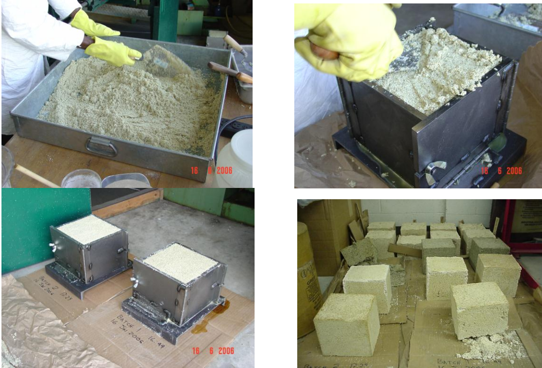
Figure 4 Kenaf Fiber Processing and Block Making
