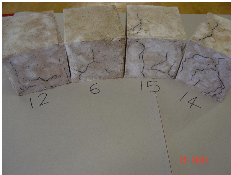
Figure 6 Kenaf Blocks Failure Patterns
