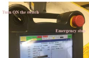
Figure 5 emergency stop on TP
