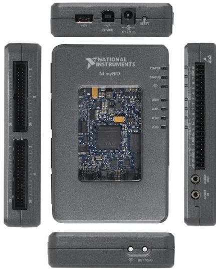
Figure 3 (a): Inputs and outputs connection of NI myRIO.
