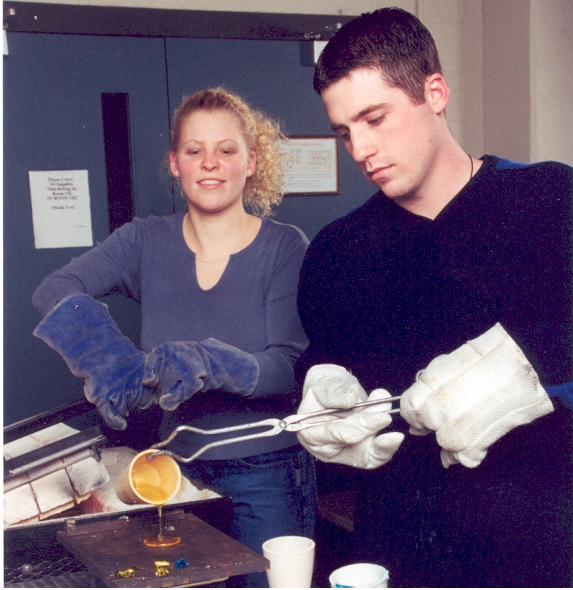
Figure 1. UMR students pouring a molten borate glass.
