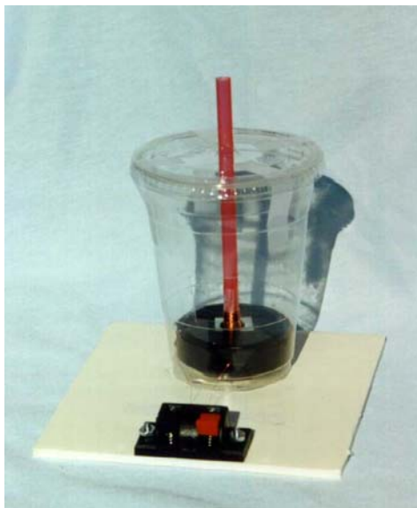
Figure 3: Electrodynamic Loudspeaker Constructed from a Plastic Cup.
