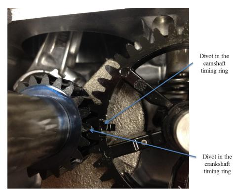
Figure 8: crankshaft timing ring aligned with camshaft timing ring
