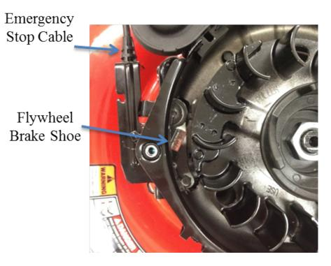
Figure 2: the emergency cable connects to the flywheel cowling and supports the flywheel brake shoe. There is also an electrical connection that stops the spark plug from firing when the handle is released.
