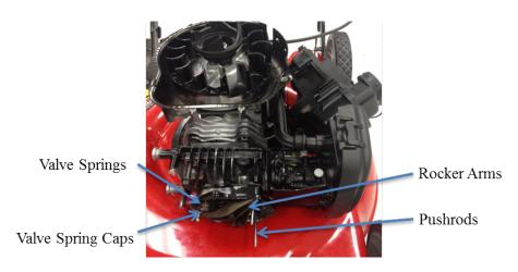
Figure 4: valve springs, rocker arms, and pushrods
