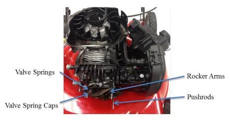
Figure 11: valve springs, rocker arms, and pushrods
