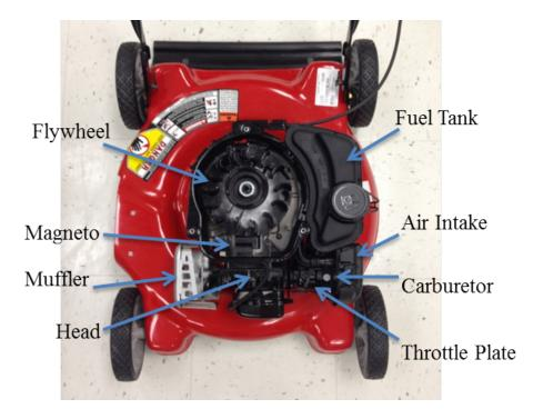
Figure 1: top view with cowling removed
