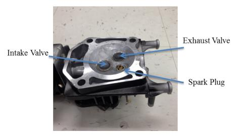
Figure 9: the cylinder head
