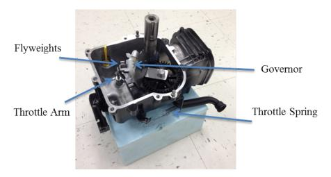
Figure 10: engine speed governing system
