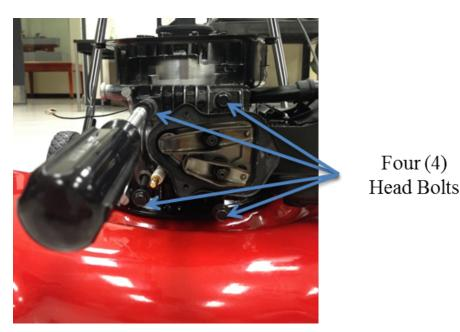
Figure 3: The four cylinder head bolts
