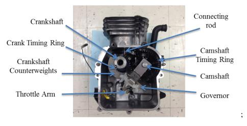
Figure 6: inside the crank case
