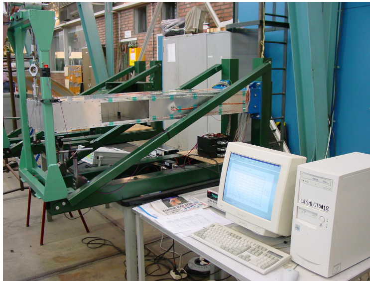
Figure 1: The wing box with a cutout in its side in the test rig
