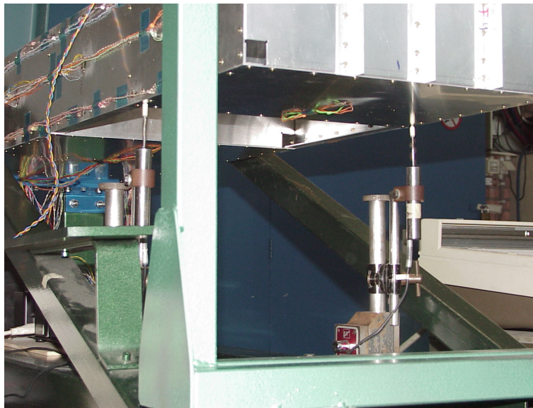
Figure 2: The wing box with a cutout in its lower side in the test rig and the linear voltage displacements transducers
