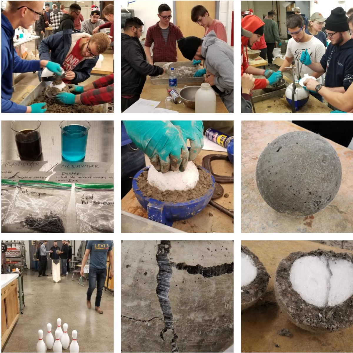
Figure 1: Students preparing and testing Concrete Bowling Ball
