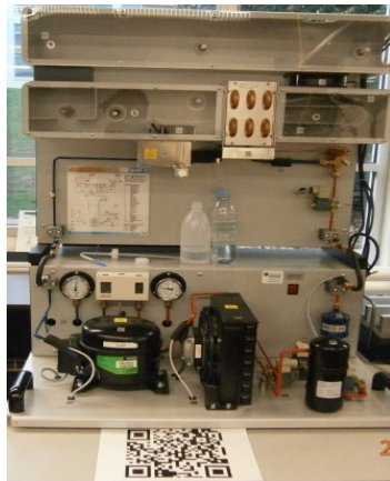
a) Refrigeration and Air conditioning unit
