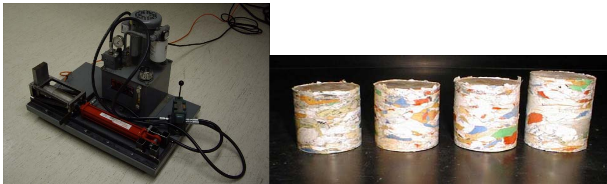
Fig.5a-5b Biomass fuel logs and compactor prototype
