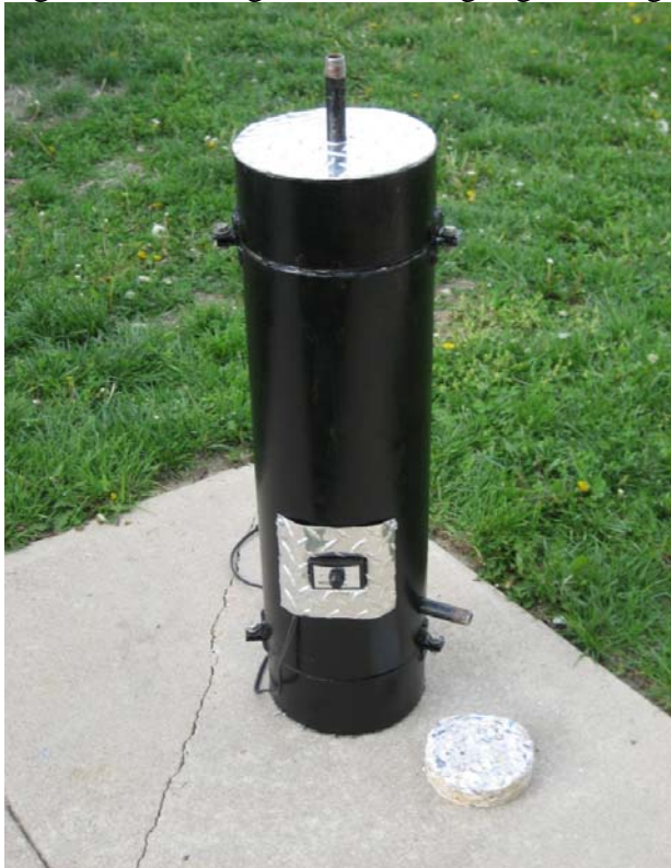
Fig.7 Prototype of a fuel gas generator using biomass logs
