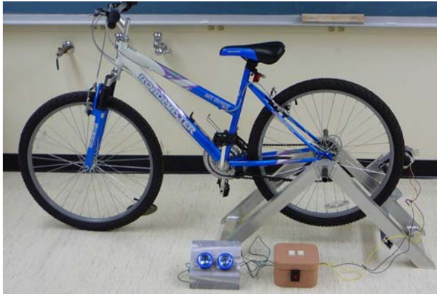
Fig.1 Generating electricity from any regular bike while exercising
