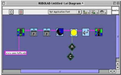
Figure 3: A simple ROBOLAB Inventor level program
