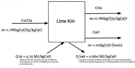
Figure 1: Material and Energy Balance for a Lime Kiln [Appendix A.1.] [4].
