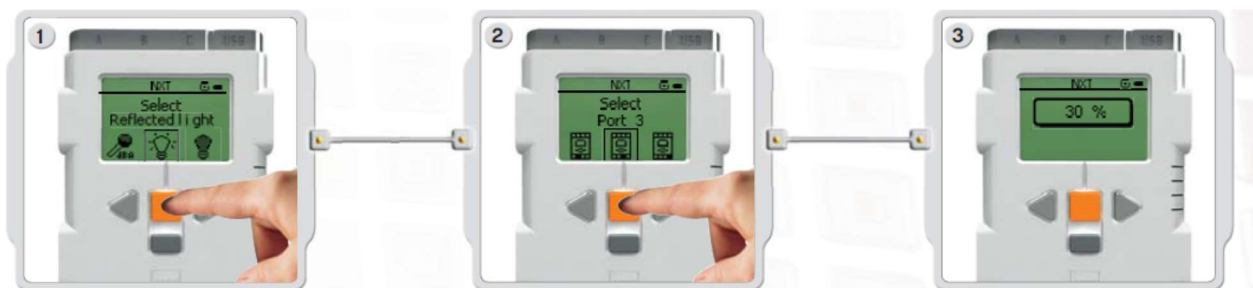
Fig. 2. The testing of light sensor's threshold setting.
