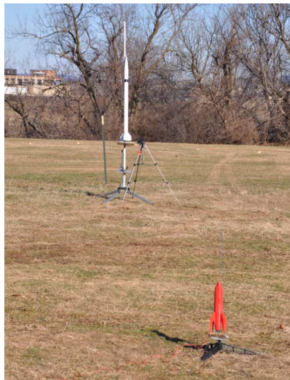
Figure 1: Two rockets await launch at the end of the semester. The black band on the large white rocket represents the location of the 3D-printed payload section and the red rocket is a fully 3D-printed rocket.
