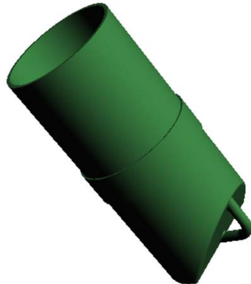
Figure 2: CAD rendering of the baseline payload section that is modified by students, 3D printed, and integrated into the Arcas model rocket.
