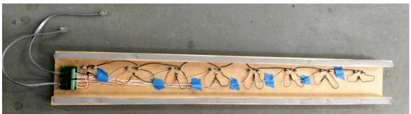
Figure 8: Piezo sensor array used in construction of MIDI enabled xylophone and glockenspiel for third part of Wild Sound. Wooden (xylophone) or metal (glockenspiel) bars are laid on sensors. The bars can either be played acoustically or their vibrations can be picked up by the piezo sensors and converted to synthesized tones.
