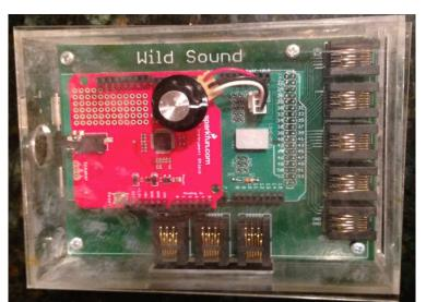
Figure 6: Wild Sound Arduino/MIDI controller and synthesizer. System is implemented as a stack of 3 circuit boards, Arduino MEGA 2560 on bottom, custom Wild Sound interface board in middle, and SparkFun Music Instrument Shield on top. A rotation encoder is used to switch between tone patches. RJ12 phone jacks provide an interface to up to 16 analog input and 34 digital input/output signals on the musical instrument control surfaces.
