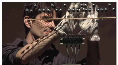
Figure 7: Clear acrylic keyboard used in performance of fourth part of Wild Sound. Conductive fabric on the fingertips of gloves worn by performers close a circuit formed with bolts and washers as keys. Standard 6 conductor phone cables connect the keyboard to the Arduino MIDI controller.
