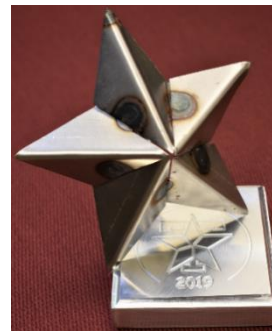
Fig. 7: Fabrication of a 3D metal star by stamping and welding.
