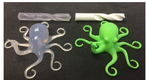
Fig. 9. Additively manufactured parts by SLA (left) and FDM (right)
