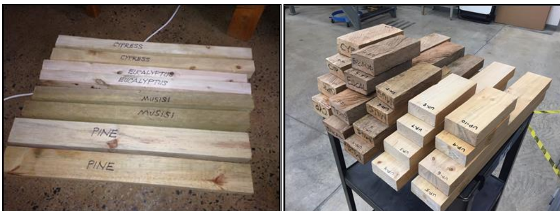
Figure 1: Wood Samples before Harvesting Specimens for Testing.
