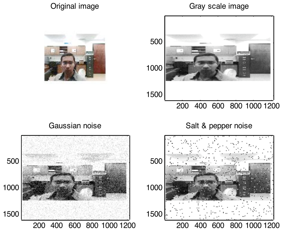
Fig. 7. Scanned version of original image (50 ppi), gray scale image of the scanned image, corrupted with Gaussian noise, corrupted with Salt & Pepper noise (clockwise).
