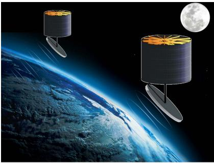
Figure 1. Solar Power Satellites (SPS) collecting sunlight in orbit and delivering Wireless Power Transfer (WPT) to terrestrial receiving antennae. This system is called Space Solar Power (SSP).
