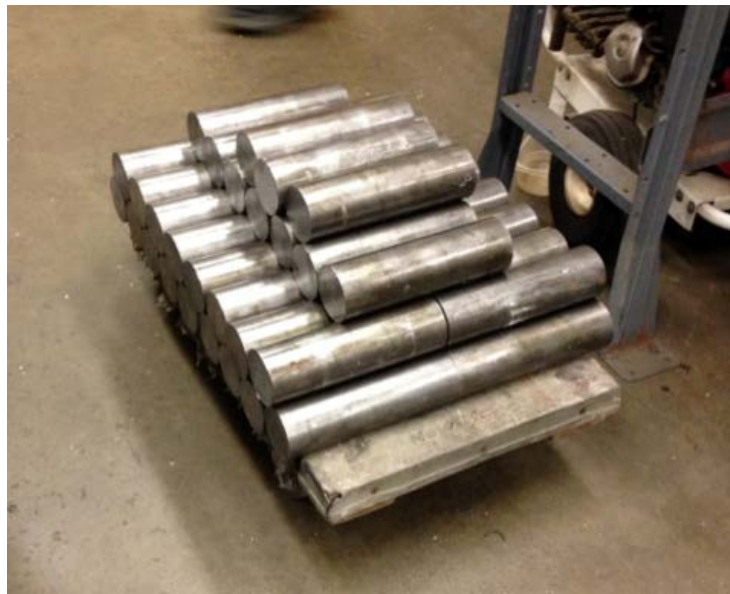
Figure 3. Incoming Raw Material (1018 Cold Rolled Steel) at $22.25/piece
