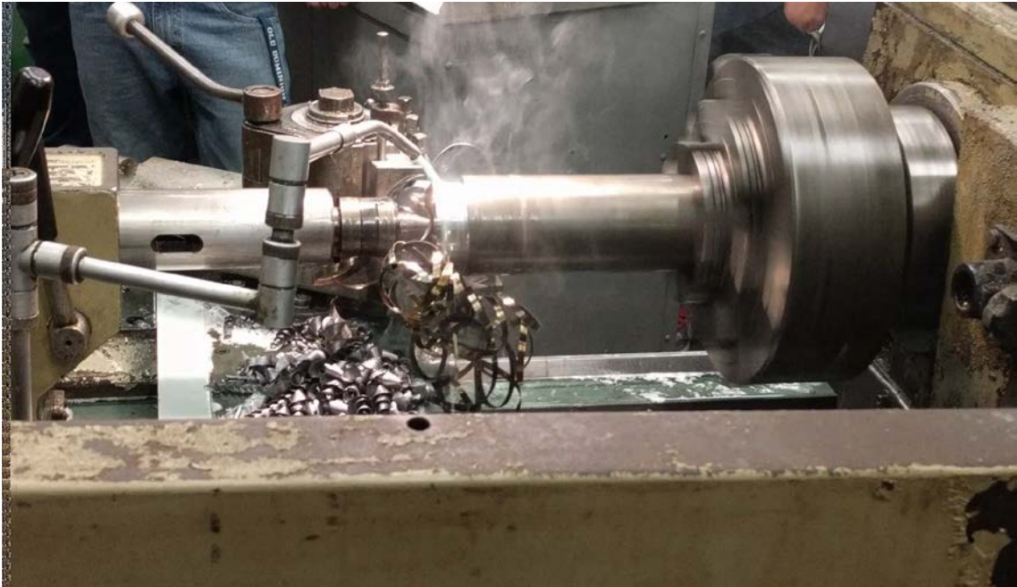
Figure A.6. Turning Operation on a Lathe
