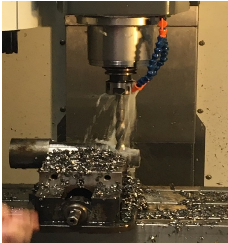
Figure A.8. Milling and Drilling Operations on the HASS CNC Machine.
