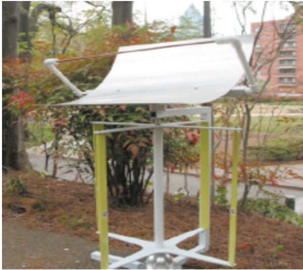
Figure 2: Concept for hybrid MRES comprising a solar PV plus concentrator heat engine and a vertical axis wind turbine.
