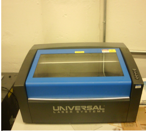
Figure 3: Benchtop CO 2 laser cutter for prototyping microfluidic chips.
