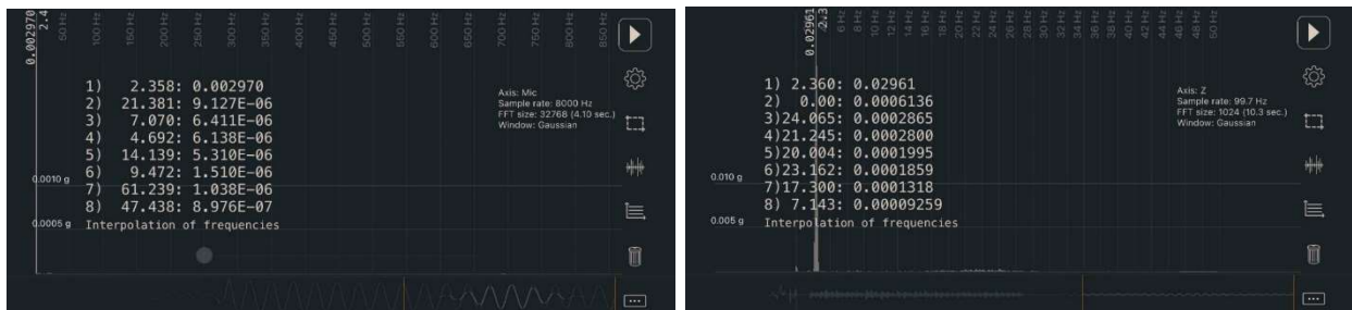
Figure 2. Vibration Analysis frequency spectra for the PCB system (left) and on-board accelerometer (right).
