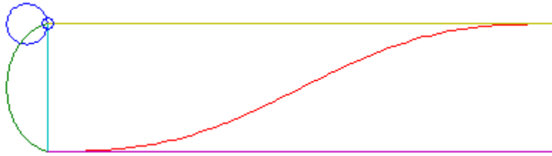
Figure 21 Cycloidal Displacement of a Cam
