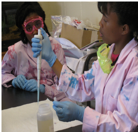
Figure 3: Participants learn to properly pipette contaminated water into microtubes to be tested for E Coli.
