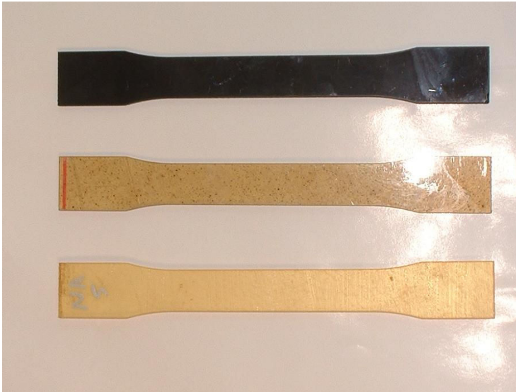
Figure 5. Test specimens with various concentrations of carbon nano tubes.
