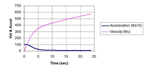
Figure 7 – Rocket velocity and acceleration
