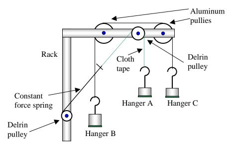
Figure 3 – Demonstration set-up for mass-weight concept
