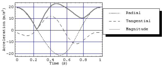
**Figure 6 – Particle tracking accelerations**
