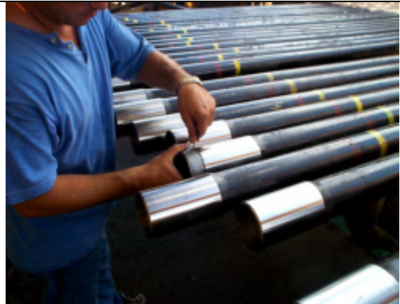
Figure 2: Conventional means of manually checking parts with thread gauges.
