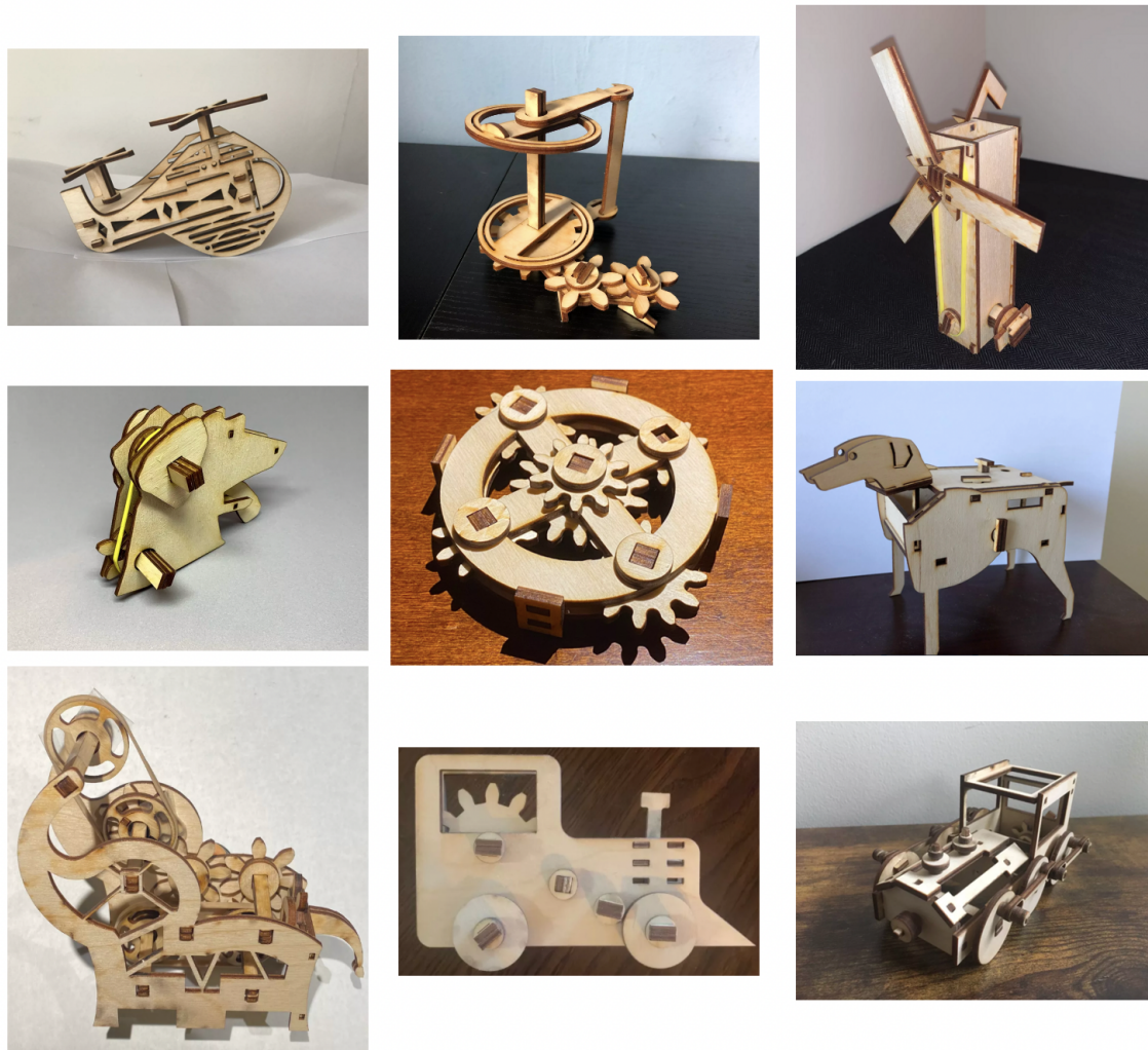
Figure 3. Final prototypes of UDGears designs in the online-only, large-enrollment FYE engineering course in Fall 2020. All designs were laser-cut using university-owned equipment and mailed to students for final assembly and testing.
