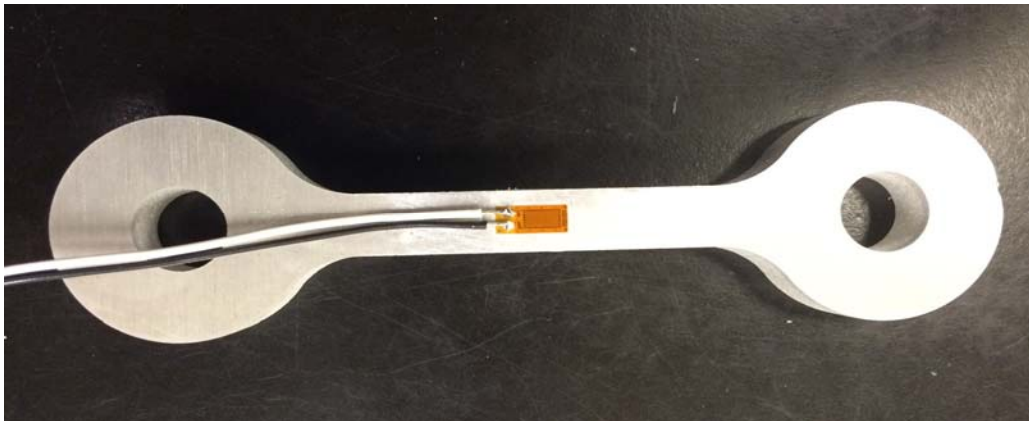
Figure 2. Students attach a strain gage to an aluminum dog-bone and solder wires to the leads.
