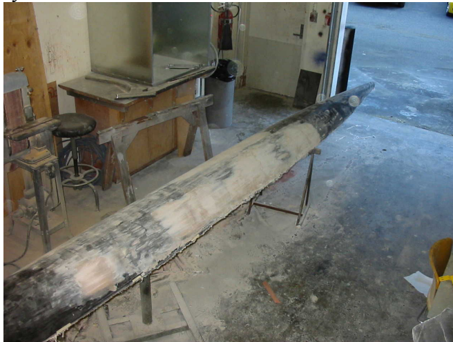
Figure 14. Shaping the splash plug.
