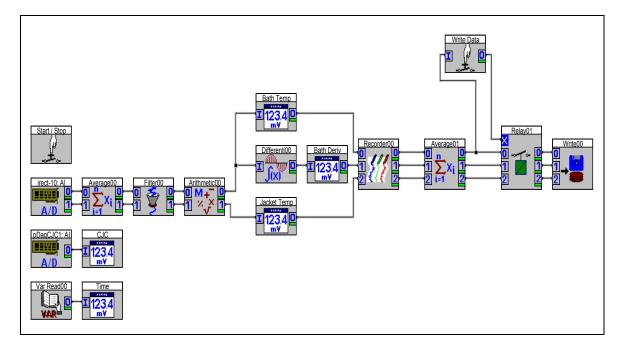
Figure 2 Data Acquisition System Block Diagram
