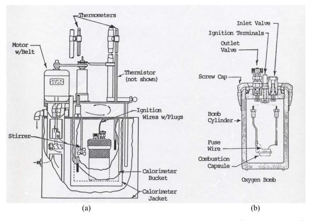
Figure 1 Schematic Diagram Showing (a) Calorimeter Cross-section<sup>3</sup> (b) Oxygen Bomb<sup>2</sup>
