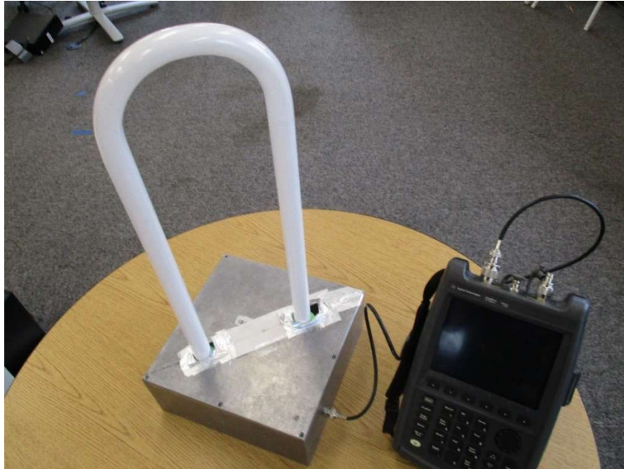
Figure 1. Plasma antenna using fluorescent tube with 122 MHz signal source.
