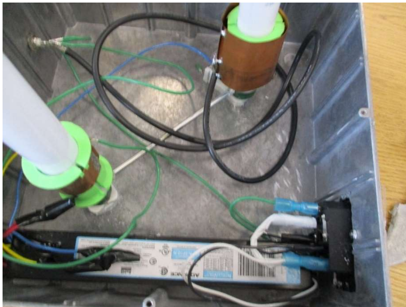
Figure 2. Construction details of plasma antenna showing 50 kHz ballast transformer and how the RF source is capacitively coupled to the gas tube via a copper rings. The leftmost ring is grounded and the right most ring receives the RF energy via the coaxial center conductor.
