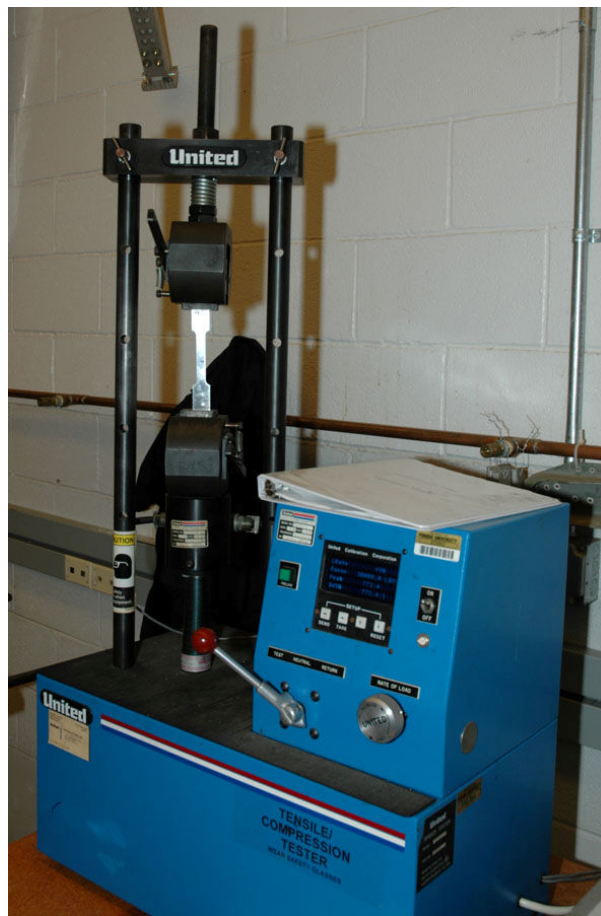
Figure 3: “Dog bone” sample in the tester.
