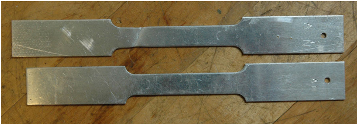
Figure 2: “Dog bone” samples before and after testing.
