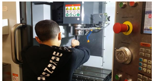
Fig 2: Student tightening the vice on the CNC milling machine after inserting the workpiece
