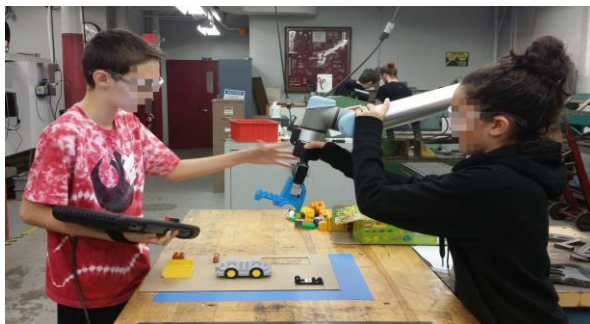
Fig 1: Students working together to program the cobot to complete the truck assembly task
