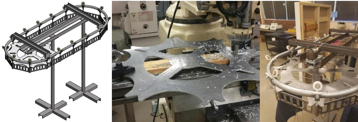
Figure 2. Intelligent Closet 3D Assembly, gear fabrication process and finished the first prototype.
