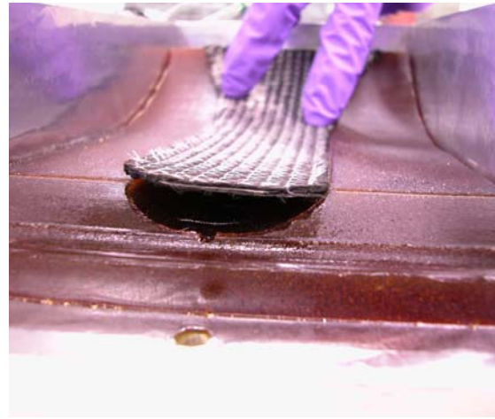
Figure 2 - Laying up carbon fiber over silicone-rubber mold
