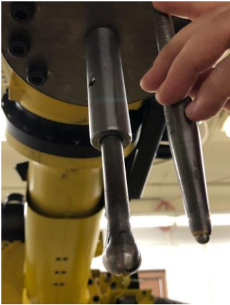
Figure 6: Side by side comparison of bigger tool (left) used in set #2 parameters versus smaller tool (right) used in set#1 parameters.
