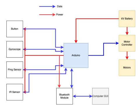
The robot will start when commanded via Bluetooth, follow the lines of a "field" based on IR data, and stop when it sees an object or when the button is pressed or when commanded by the GUI. It will collect and send data that can be displayed by the GUI when requested and all data will be saved to a csv file. There are multiple hardware subcircuits that have to be included without exceeding the current load for the Arduino.
