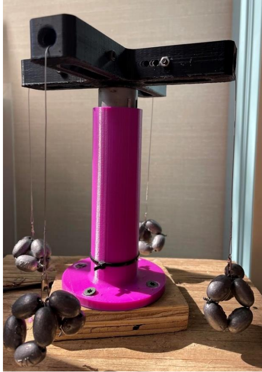
Figure 4: Group 2's carousel (with adjustable cable and motor inside)
