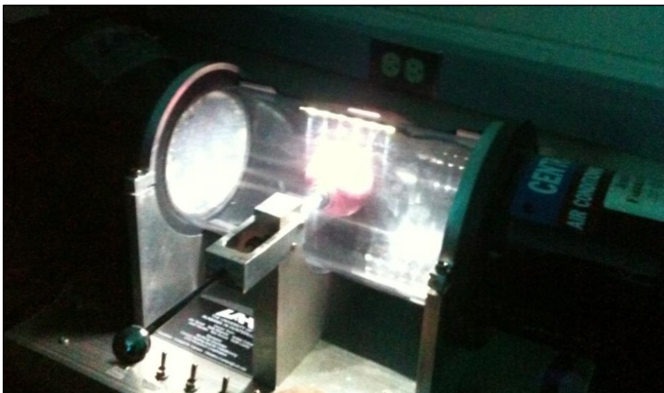
Figure 7. Test section of the Phase III wind tunnel showing visible laminar streamlines upstream (left) of the spherical test article and turbulent flow downstream (right) of the test article ( photo credit: C. Carmen )
