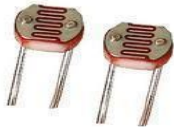
Figure 5. Small photoresistors that have a resistance of 10\text{K ohms} .
