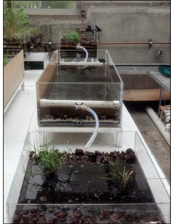
Figure 9: Final free water surface system
