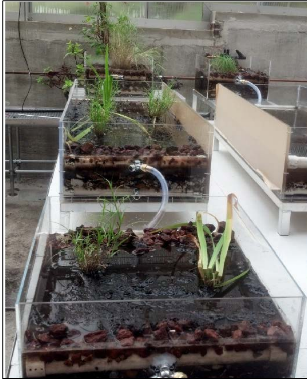
Figure 8: Final subsurface system
