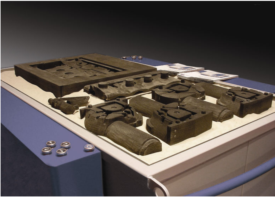
Figure 3. Core and Mold Parts Made Simultaneously in a Single Cavity (Courtesy of ProMetal, a division of the Ex One Corporation)
