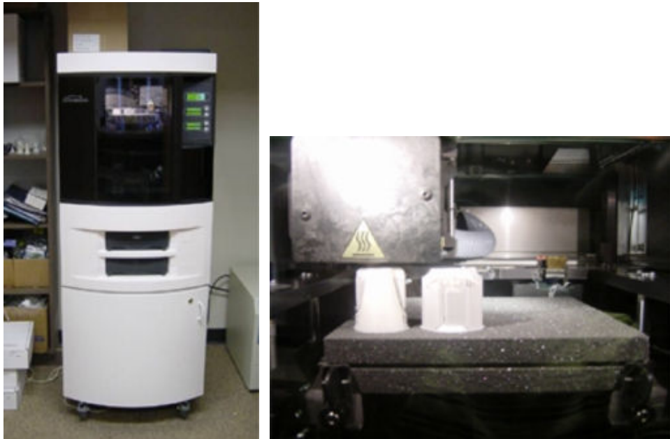
Figures 3 and 4: Penn State Altoona's Dimension FDM machine and view of build in progress
