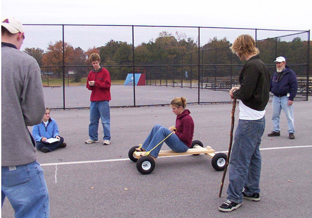
Figure 6—Collecting data to determine the change in velocity of the downhill racer when rolling down the sloped asphalt
