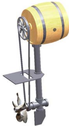
Figure 2. Belt Drive and Wood Barrel Covering the Electric Motor
