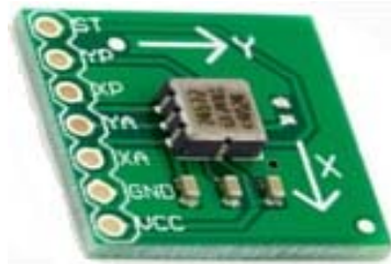
Fig. 1: ADXL203CE accelerometer and breakout board
