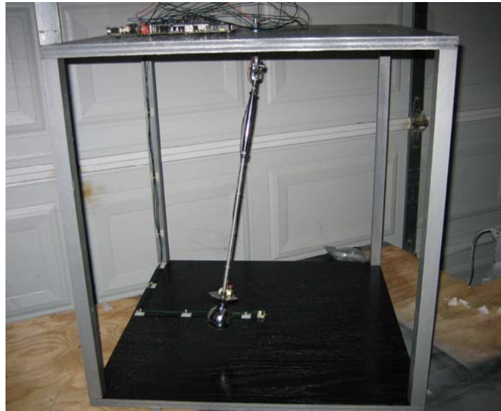
Fig. 3: measurement of pendulum acceleration
